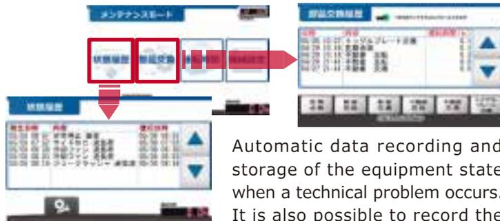
Automatic data recording and storage of the equipment state when a technical problem occurs. It is also possible to record the replacement time of each spare part, to improve servicing and schedule downtime maintenance.
