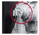
the crushing chamber, it will be discharged using the hydraulic assist device.Not only the protection of the electric motor, but also the restoration of work can be done safely in a short period of time.
