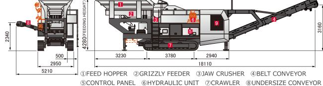
©CONTROL PANEL ©HYDRAULIC UNIT ©CRAWLER ®UNDERSIZE CONVEYO ®DIESEL GENERATOR (Option)
