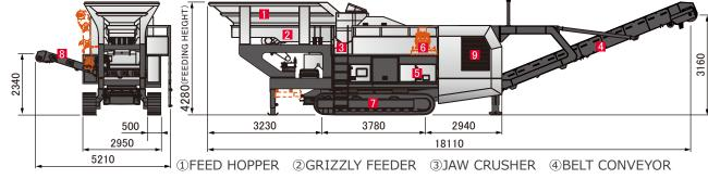
©CONTROL PANEL ©HYDRAULIC UNIT ©CRAWLER @UNDERSIZE CONVEYOR
