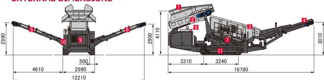
①FEED HOPPER ②APRON FEEDER ③VIBRATING SCREEN ④OVERSIZE CONVEYOR ⑤UNDERSIZE CONVEYOR **(II)CONTROL PANEL (II)CRAWLER**
