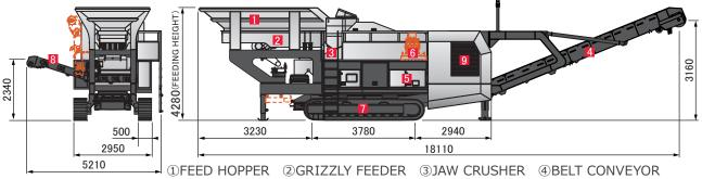
→ ①FEED HOPPER ②GRIZZLY FEEDER ③JAW CRUSHER ④BELT CONVEYOR ⑤CONTROL PANEL ⑥HYDRAULIC UNIT ⑦CRAWLER ⑧UNDERSIZE CONVEYOR ⑨DIESEL GENERATOR (Option)
