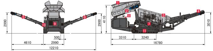
①FEED HOPPER ②APRON FEEDER ③VIBRATING SCREEN ④OVERSIZE CONVEYOR ⑤UNDERSIZE CONVEYOR
