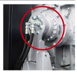
the crushing chamber, it will be discharged using the hydraulic assist device. Not only the protection of the electric motor, but also the restoration of work can be done safely in a short period of time.
