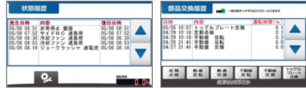
Automatic data recording and storage of the equipment state when a technical problem occurs. It is also possible to record the replacement time of each spare part, to improve servicing and schedule downtime maintenance.
