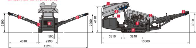
①FEED HOPPER ②APRON FEEDER ③VIBRATING SCREEN ④OVERSIZE CONVEYOR ⑤UNDERSIZE CONVEYOR ⑥MIDDLESIZE CONVEYOR ⑦BELT CONVEYOR ⑧DIESEL GENERATOR ⑨HYDRAULIC UNIT ⑩CONTROL PANEL ⑪CRAWLER
